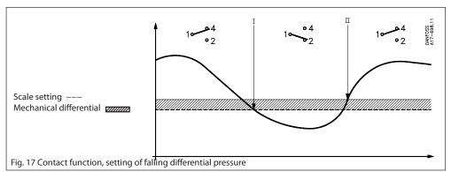
b. Units with adjustable neutral zone (SPDTNP) If the differential pressure rises above the set value plus the differential, contacts 1-4 make. If the pressure falls by the amount of the differential (which is fixed in this unit), contacts 1-4 break. If the pressure falls to the neutral zone minus the differential, contacts 1-2 make. When the differential pressure rises again by an amount corresponding to the differential, contacts 1-2 break again.
