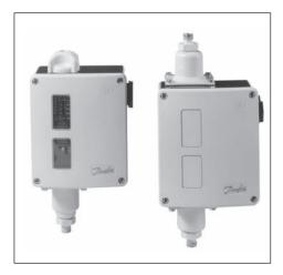
Type RT pressure switches incorporate a pressure controlled, single-pole changeover switch where the contact position depends on the pressure in the connection port and the set value. The RT series consists of pressure switches, differential pressure switches and pressure switches for neutral zone regulation. These units are for general use within the industrial and marine sectors.
