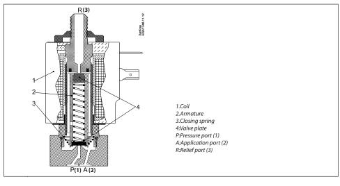
*Coil voltage disconnected (closed):*
