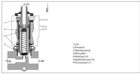
Coil voltage disconnected (open): When the voltage is disconnected, the armature (2) with the valve plates (4) is pressed down by the opening spring (3) and closes the connection between A and R. At the same time, the connection between ports P and A is open. The connection between P and A will be open for as long as the voltage to the coil is disconnected. On valves with manual override the connection between P and A can be closed using a closing screw in the valve body.
