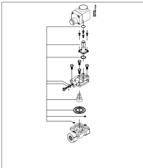
The kit comprises a O-ring for coil, Armature unit assembly, O-ring for the armature unit, spring and diaphragm, two O-rings for the pilot system, and an O-ring and gasket for the equalising orifice.
