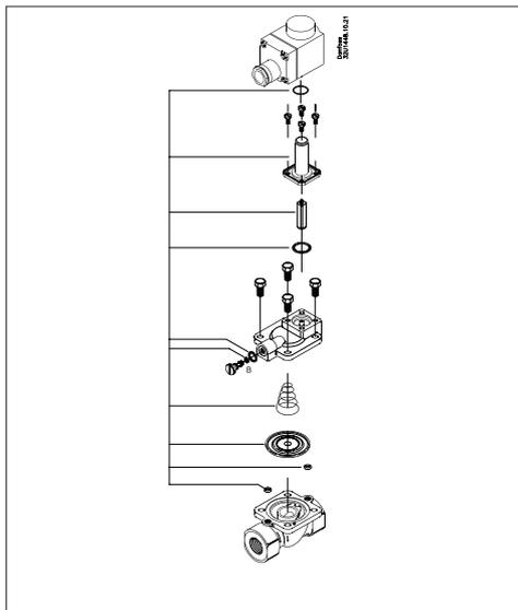
The kit comprises a O-ring for coil, armature with valve plate and spring, O-ring for the armature tube, spring and diaphragm, two O-rings for the pilot system, and an O-ring and gasket for the equalising orifice.
