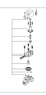
The kit comprises a O-ring for coil, armature with valve plate and spring, O-ring for the armature tube, spring and diaphragm, two O-rings for the pilot system, and an O-ring and gasket for the equalising orifice.
