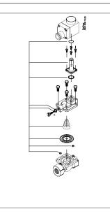
The kit comprises a O-ring for coil, Armature unit assembly, O-ring for the armature unit, spring and diaphragm, two O-rings for the pilot system, and an O-ring and gasket for the equalising orifice.
