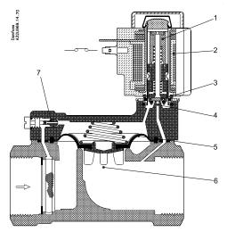
5.Diaphragm 1.Armature 2.Coil 6.Main orifice 3. Valve plate 7. Equalising orifice 4.Pilot orifice
